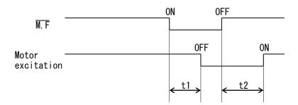
$t1 \le 5ms$  (t1: Time required for the motor output current to be shut off.)
