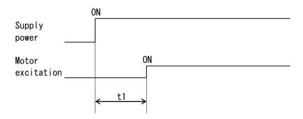
$t1 \le 300ms$  (t1: Time required for the motor to be enabled.)
