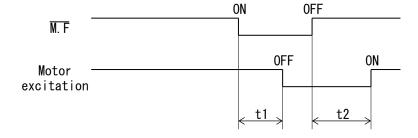
$t1 \le 5ms$  (t1: Time required for the motor output current to be shut off.)
