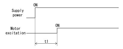
$t1 \le 1s$  (t1: Time required for the motor to be enabled.)
