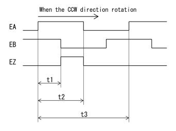
$t1 \ge 1.25 \,\mu$ s,  $t2 \ge 2.5 \,\mu$ s,  $t3 \ge 5 \,\mu$ s Maximum response frequency : 200kHz
