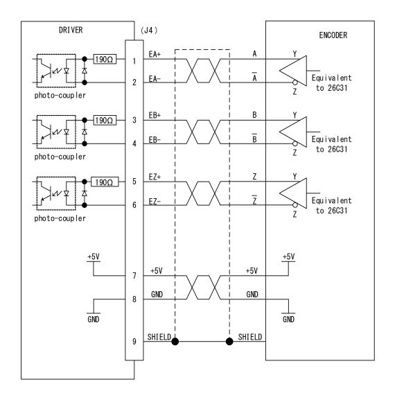
● +5V and GND are not insulated from the internal power supply of the DRIVER.
