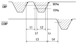
$t1 \ge 2 \mu s$ ,  $t2 \ge 2 \mu s$ ,  $tf, tr \le 2 \mu s$  $t3 \ge 4 \mu s$ ,  $t4 > 4 \mu s$  Maximum response frequency : 250kHz
