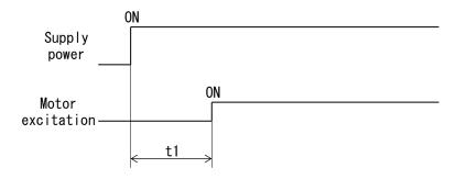
$t1 \le 1s$  (t1: Time required for the motor to be enabled.)
