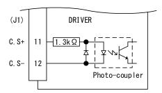
Step angle division is switched to 2 or 5 divisions of the basic angle with the photo-coupler ON.
