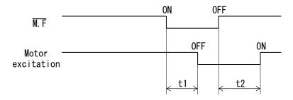
t1≦5ms (t1: Time required for the motor output current to be shut off.)
