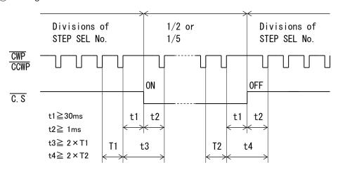
Switching the step angle by the C.S signal requires time "t1", "t2", "t3" and "t4" before and after inputting drive pulse.
