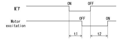
t1≤5ms (t1: Time required for the motor output current to be shut off.)
