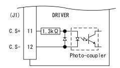
Step angle division is switched to 20 divisions of the basic angle with the photo-coupler ON.
