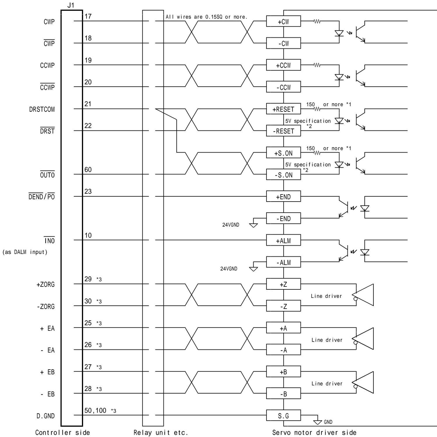
\*1 If the current limiting resistor on the driver side is less than 150 Ω, externally add resistor so that the total resistor value becomes 150 Ω or more.
