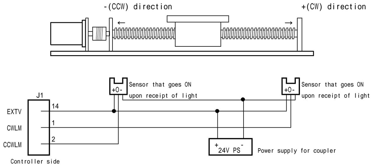
• The initial value of the limit signal is active-off (B contact) input.
