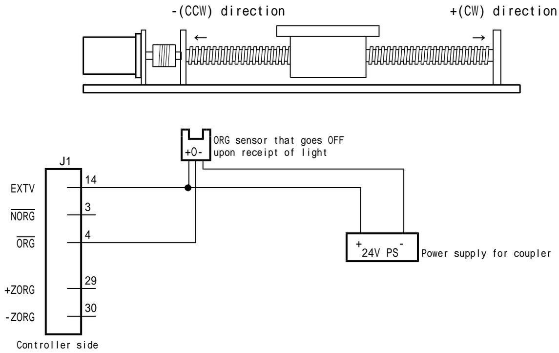
**When using the origin sensor+origin proximity signal**
