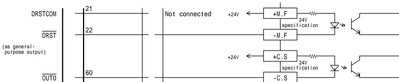
\*3 The signal is connected when the encoder is used.
