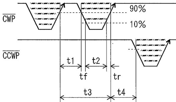
$t1 \geq 1\mu\text{s}$ ,  $t2 \geq 1\mu\text{s}$ ,  $t_f, t_r \leq 2\mu\text{s}$
